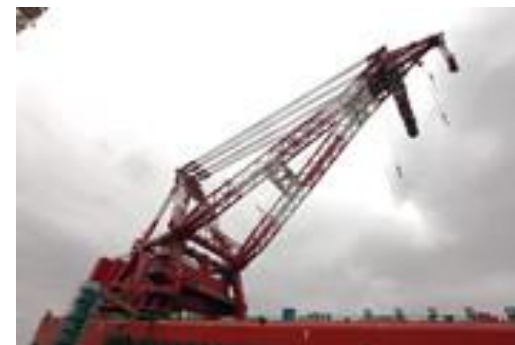
The world's largest floating crane -- 12,000 ton self-propelled revolving floating crane
