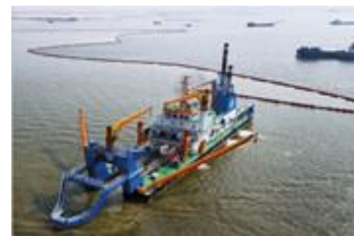
The working cutter suction dredger and the dredging pipe line
