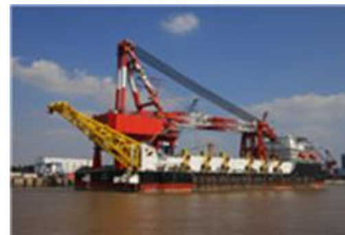
3,000 ton shallow pipe-laying vessel
