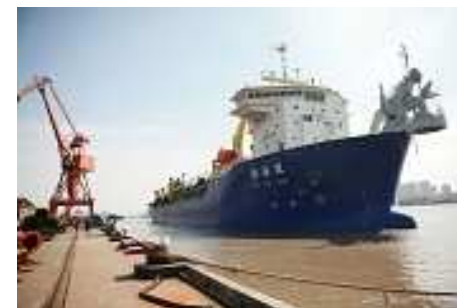
“Xin Hai Feng”, Self-propelled trailing suction hopper dredger, participated in Brazil’s dredging project
