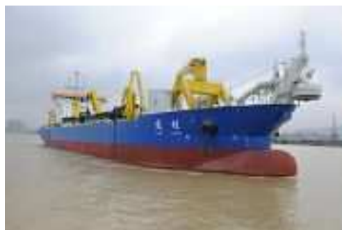
“Tong Cheng”, self-propelled trailing suction hopper dredger with the largest tank capacity and deepest digging depth in the PRC
