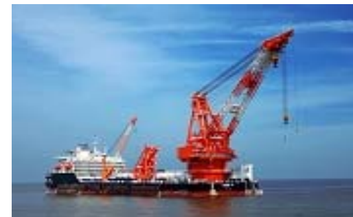
A 1200t pipe laying vessel designed and built by ZPMC
