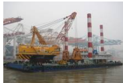
“Xin Hai Bang”, a 27 square metre clamshell dredger researched and developed by CCCC and built by ZPMC
