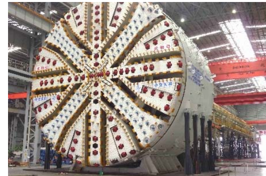
Tunnel Boring Machine manufactured by CCC
